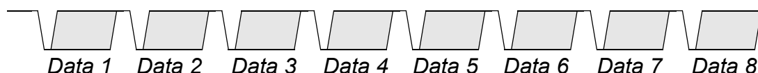
Figure 2.8: Numbering of the data bytes in a frame with eight data bytes.
